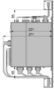
The left-hand side of the unit heat sink is fastened to a metal wall using 2 retaining plates.
